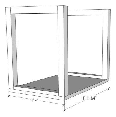
3. Next, add shelf support at desired height. I attached mine with a 2" space in between as I'm only storing mats here.
