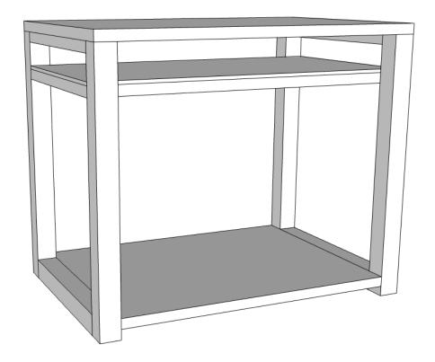
7. If adding a vinyl holder, attach 1x4 at one end using pocket hole screws. As shown here, 1x4 is 14 ¼" long, but this will depend on how you installed bottom shelf. If your middle shelf is lower, you may need to cut your 1x4 in half and attach 1 part above and one part below.
